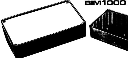
The BIM 1000 range of small desk consoles is manufactured in ABS and is fitted with 1mm (.04") thick grey aluminium front panels which drop into the sloping front of the consoles and held by four fixing screws running into integral brass bushes.
