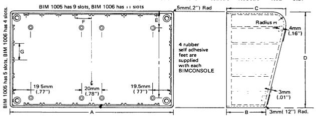
Note All side walls are nominally 2 5mm( 1") thick between 1.8mm( 07") wide, 1mm(.04") deep pcb slots.
