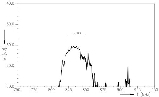
Frequency Response TX-RX (Wideband Common Mode Isolation)
