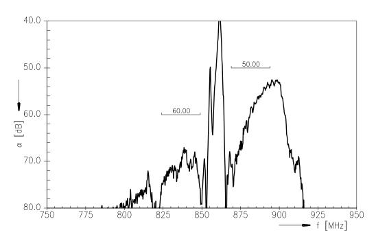
Frequency Response TX-RX (Wideband Differential Mode Isolation)
