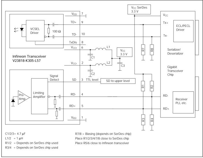
Values of R1/2/3/4 may vary as long as proper 50  $\Omega$  termination to  $V_{EE}$  or 100  $\Omega$  differential is provided. The power supply filtering is  $\,$  required for good EMI performance. Use short tracks from the inductor L1/L2 to the module  $V_{CC}Rx/V_{CC}Tx$ .
