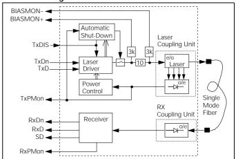
The receiver component converts the optical serial data into PECL compatible electrical data (RxD and RxDn). The Signal Detect (SD, active high) shows whether an optical signal is present<sup>(1)</sup>.
