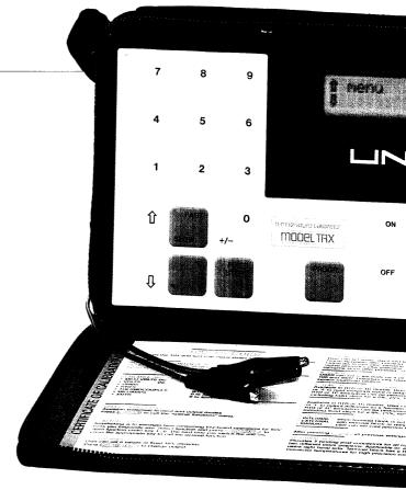
"switch-on" preference can be set by the user. Up to six output values for each type of signal can be temporarily stored and recalled manually or automatically (auto-stepping). Step timer setting is adjustable from 10 to 100 seconds.
