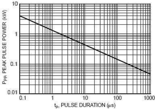
Figure 1. Non-Repetitive Peak Pulse Power versus Pulse Time
