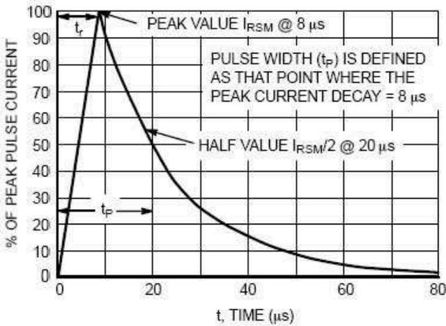
Figure 3.  $8 \times 20 \mu\text{s}$  Pulse Waveform
