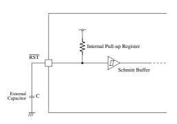
A  $0.01\mu F$  external capacitor is recommended. However, the time constant can be lengthened if longer time is required for the XTI and LRCI clocks to stabilize after power-ON.
