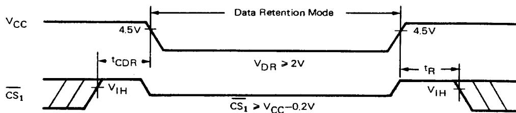
Low  $V_{CC}$  Data Retention Waveform (2) ( $\overline{CS}_2$  Controlled)
