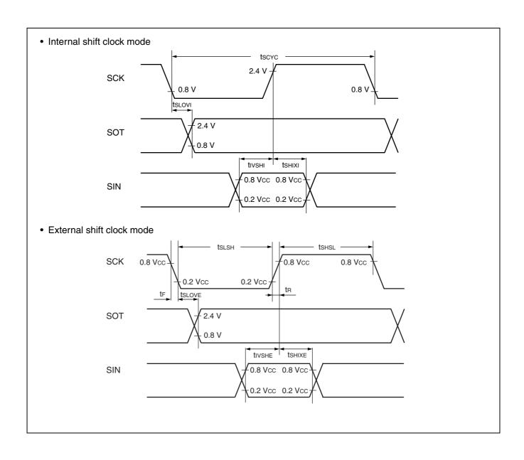
Sampling at the falling edge of sampling clock<sup>1</sup> and prohibited serial clock delay<sup>2</sup>
