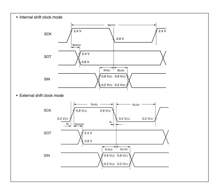
Sampling at the rising edge of sampling clock<sup>1</sup> and enabled serial clock delay<sup>2</sup>
