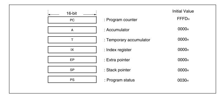
The PS can further be divided into higher 8 bits for use as a register bank pointer (RP) and a direct bank pointer (DP) and the lower 8 bits for use as a condition code register (CCR). (Refer to the diagram below.)
