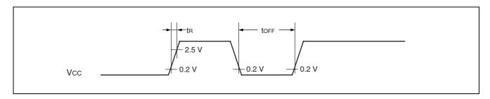
Note: Sudden change of power supply voltage may activate the power-on reset function. When changing power supply voltages during operation, set the slope of rising within 30 mV/ms as shown below
