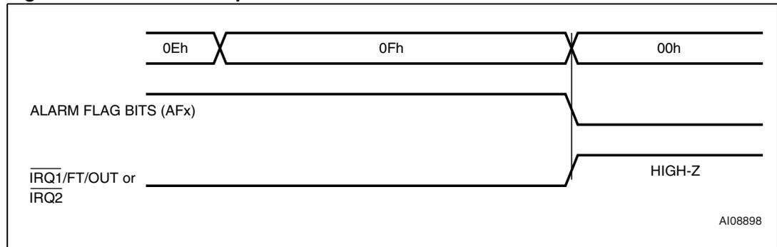
**Figure 22. Back-up mode alarm waveform**
