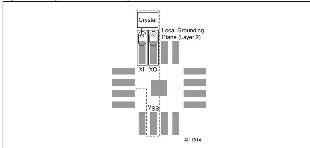
1. Substrate pad should be tied to  $V_{SS}$ .
