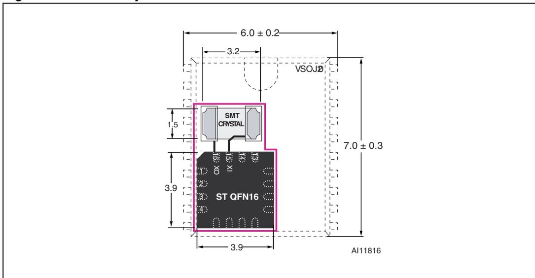
1. Dimensions shown are in millimeters (mm).
