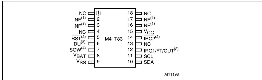
1. NF pins must be tied to VSS. Pins 2 and 3, and 16 and 17 are internally shorted together.
