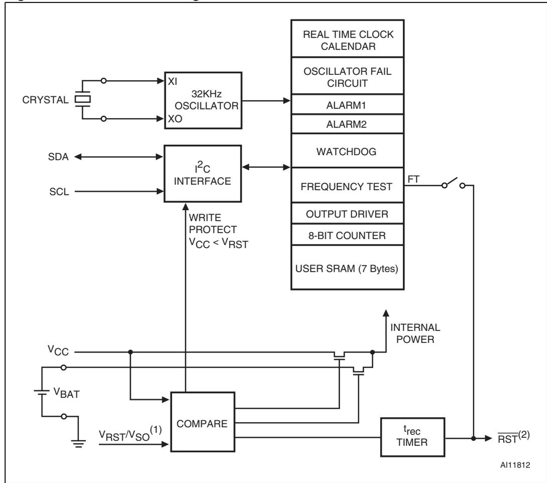
1.  $V_{RST} = V_{SO} = 2.93V$  (S), 2.63V (R), and 2.32V (Z).
