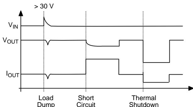
Figure 2. Typical Circuit Waveforms for Output Stage Protection
