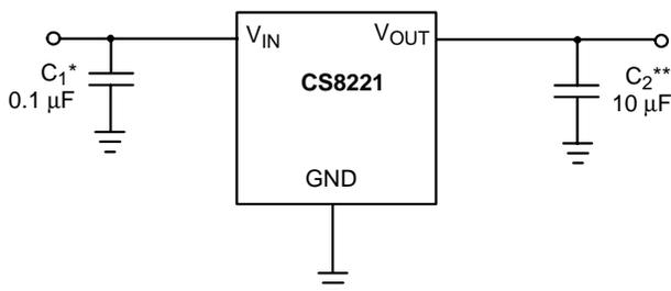
\* $C_1$  is required if regulator is far from the power source filter.
