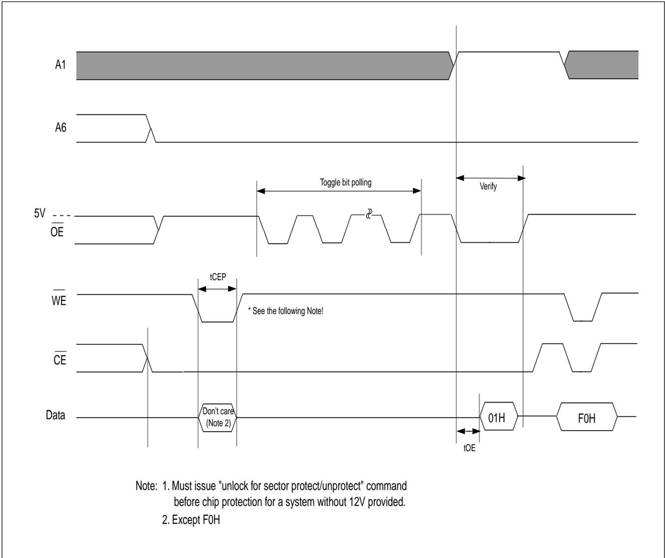
**TIMING WAVEFORM FOR CHIP UNPROTECTION FOR SYSTEM WITHOUT 12V**
