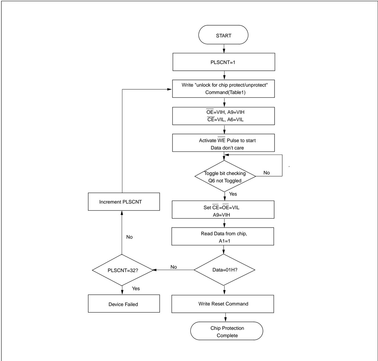
**CHIP UNPROTECTION ALGORITHM FOR SYSTEM WITHOUT 12V**
