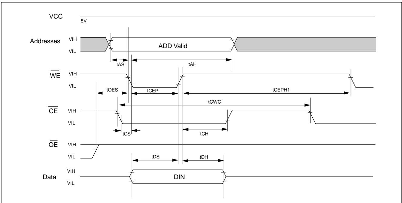
**AUTOMATIC PROGRAMMING TIMING WAVEFORM**
