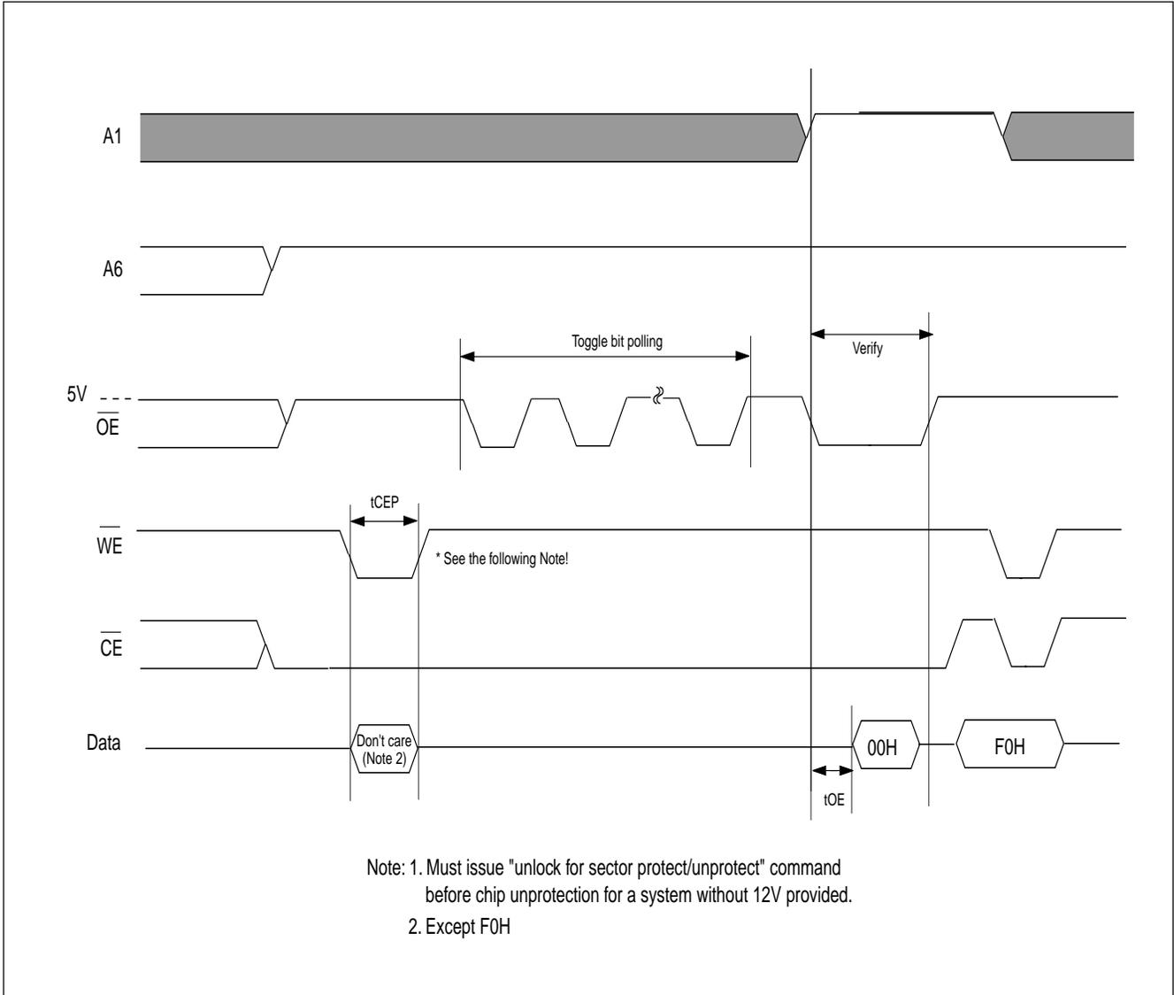
**CHIP PROTECTION ALGORITHM FOR SYSTEM WITHOUT 12V**
