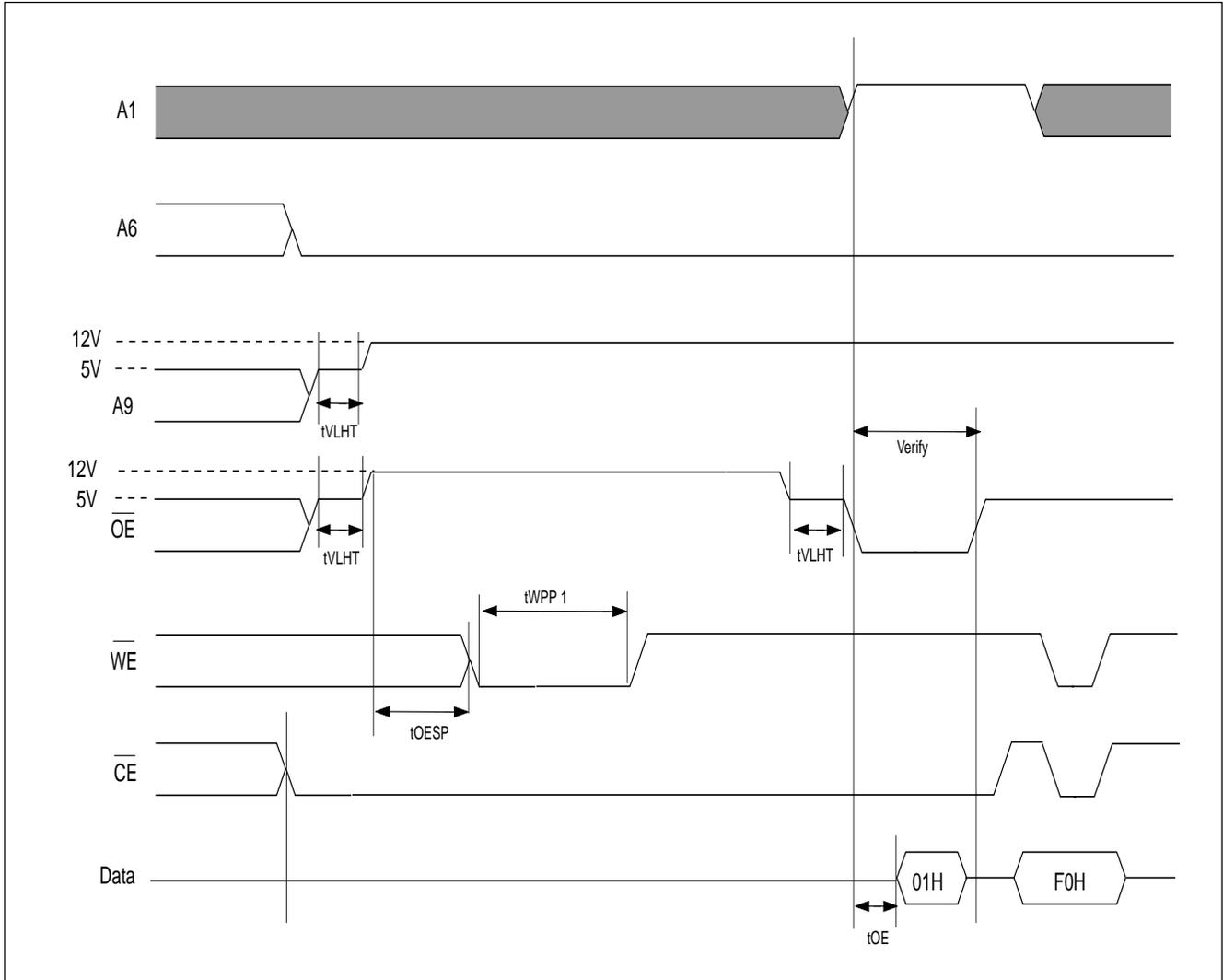
**TIMING WAVEFORM FOR CHIP UNPROTECTION FOR SYSTEM WITH 12V**
