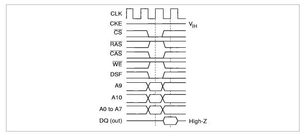
**Column address and write command:** For a row of one of two banks activated by ACTV or ACTVM, at the CLK rising edge, by setting
