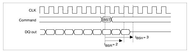
**Burst stop command at burst write:** For full page burst write cycle, when a burst stop command is issued, the write data at that cycle and the following write data input are ignored. The BST command is legitimate only in case full page burst mode, and is illegal for burst length 1, 2, 4 or 8.
