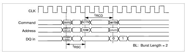
Special Mode Register Set (Load Mask) in Active State and Write Per Bit
