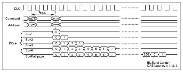
**Single write:** Before executing a single write operation, OPCODE (A10, A9, A8) should be set to (0, 1, 0). In the single write operation, data are only written to the single column defined by the column address and the bank select address loaded at the write command set cycle regardless of the defined burst length. (The latency of data input is 0).
