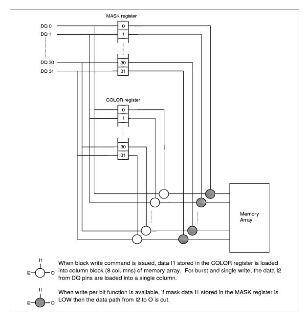
**Column address and block write command:** For a row of one of two banks activated by ACTV or ACTVM, at the CLK rising edge, by setting
