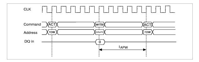
**Block write with auto-precharge:** In this operation, since precharge is automatically performed after completion of a block write operation, so no need to execute precharge command. The following command must be a bank active command (ACTV, ACTVM). In addition, an interval of  $l_{APBW}$  is required between the last valid data input and the following command.
