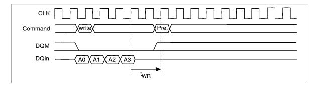
Block Write Command to Precharge Command Interval: The minimum interval between block write command and the following precharge command is  $t_{BWR}$ .
