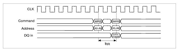
**Special Mode Register Set to Block Write/Write Interval:** The minimum interval between a special mode register set and a block write/write is  $t_{SBW}$ .
