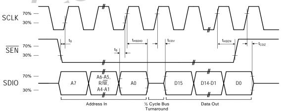
Figure 5. 3-Wire Control Interface Read Timing Parameters
