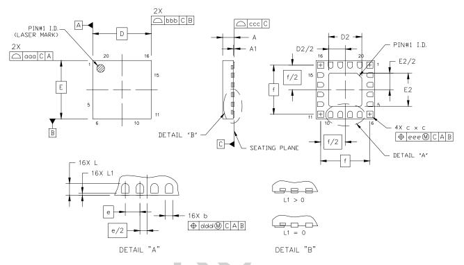
Figure 10. 20-Pin Quad Flat No-Lead (QFN)
