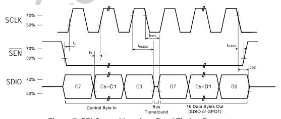
Figure 7. SPI Control Interface Read Timing Parameters
