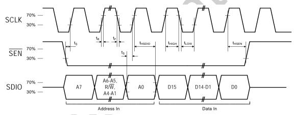
Figure 4. 3-Wire Control Interface Write Timing Parameters
