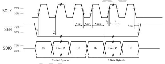
Figure 6. SPI Control Interface Write Timing Parameters
