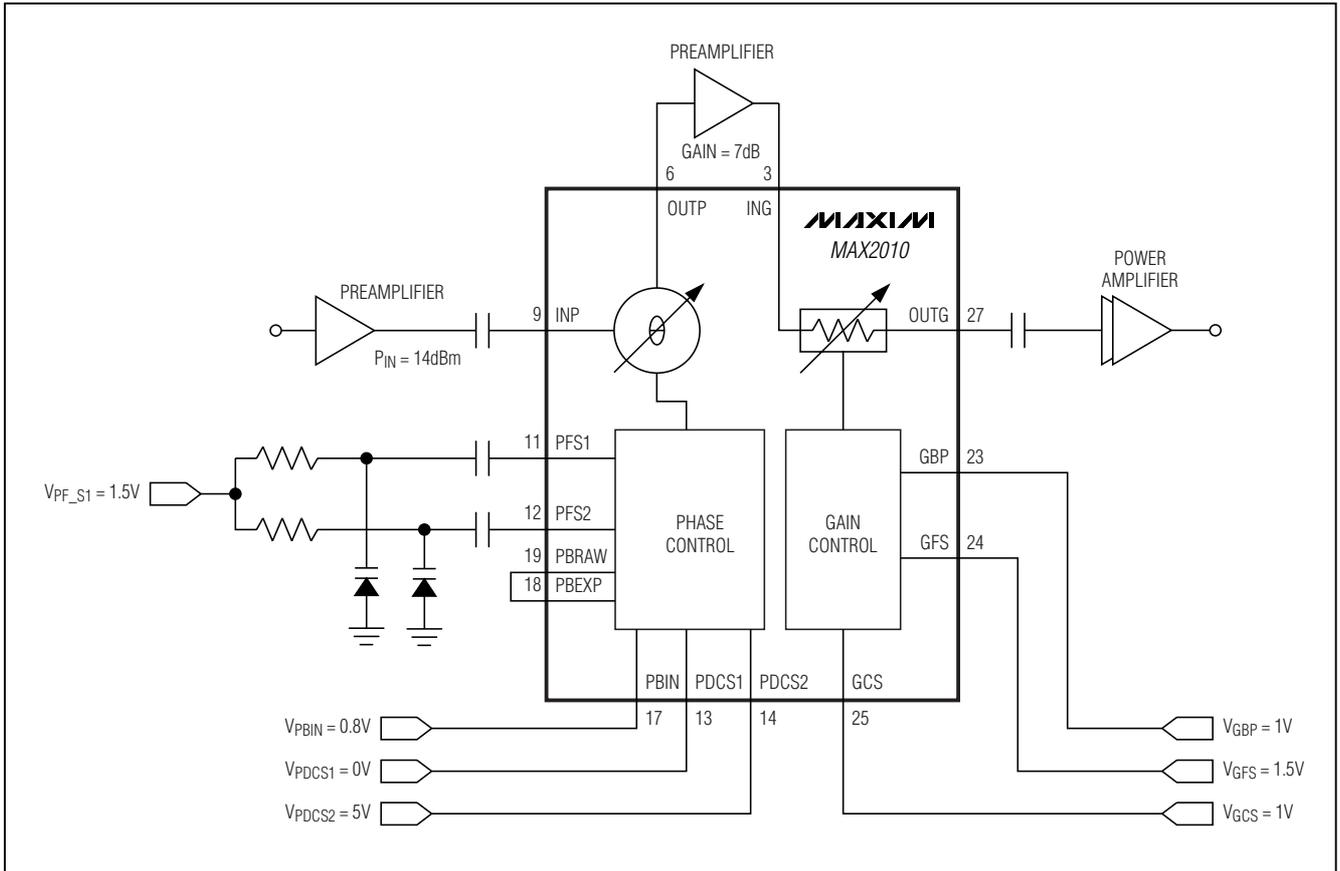
Figure 5. MAX2010 Phase and Gain Optimization Circuit
