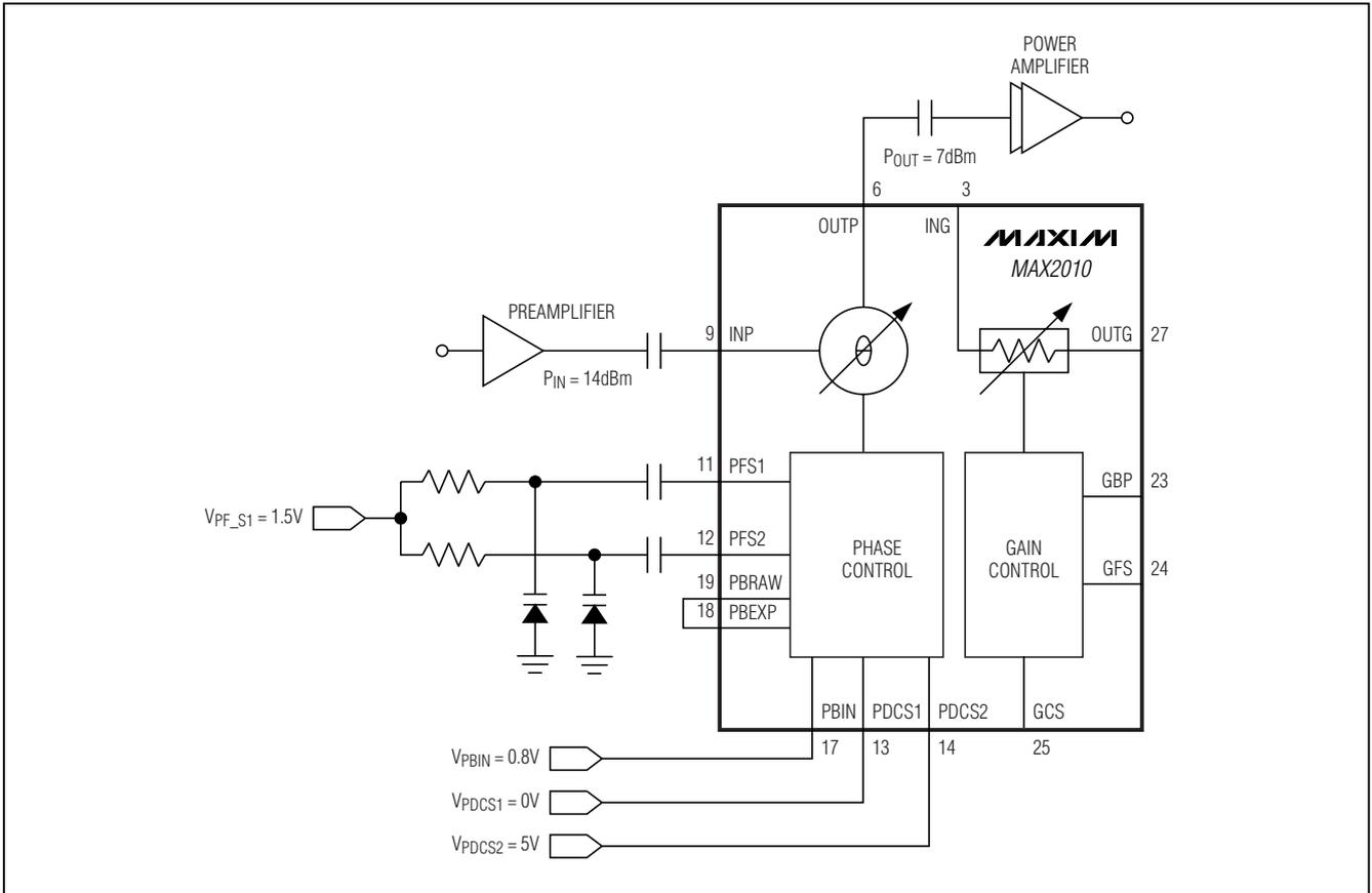
Figure 4. AM-PM Response Tuning Circuit
