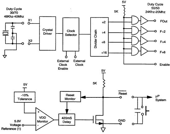
(1) Without a 5.0V reference supplied to pin 1, the supply voltage monitoring function is disabled.
