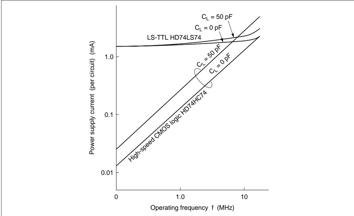
**Figure 13 Operating Frequency vs Power Supply Current**
