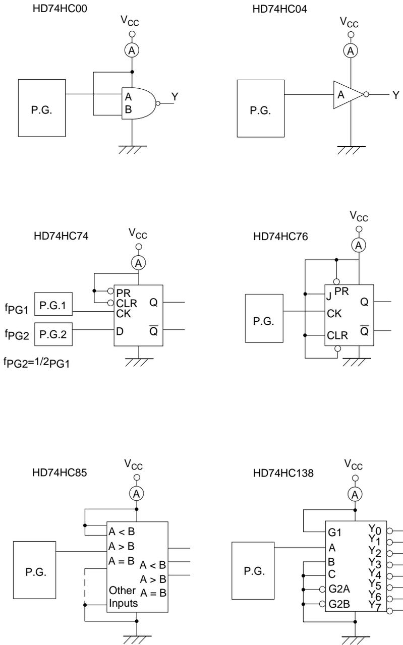
**Figure 14 Measurement Circuits for Dynamic Power Supply Current**
