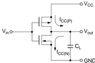
**Figure 6 Inverter circuit**
