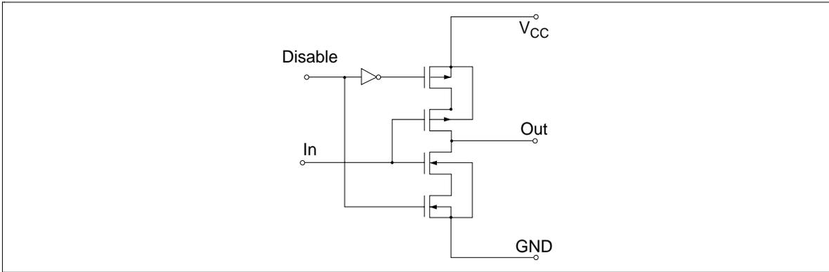
**Figure 5 3-state Output Circuit**
