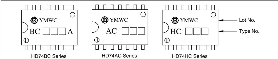
Note: Meaning of marking on package example device name:
