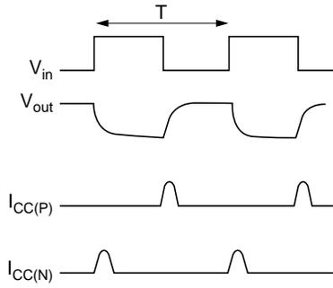
**Figure 7 Operating Voltage and current of inverter circuit**
