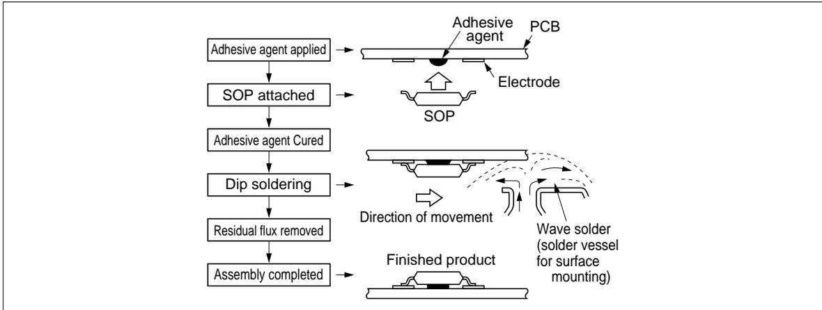
**Figure 27 Process Flow for Dip Soldering SOP**
