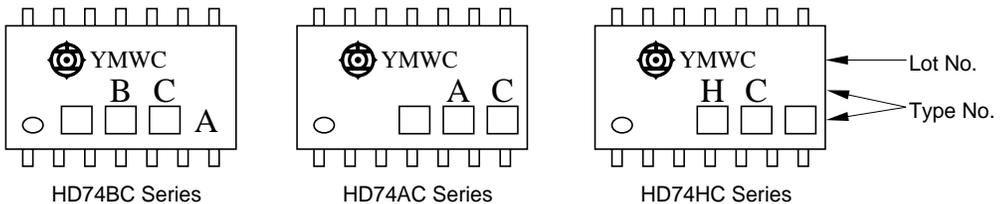
Note: Meaning of marking on package example device name:
