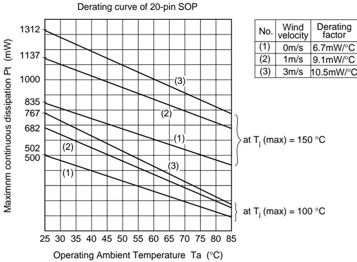
**Note:** When  $T_a$  is below  $25^\circ\text{C}$ ,  $P_T$  becomes the same value as at  $T_a = 25^\circ\text{C}$  being independent of  $T_a$ . The data above was measured by using the  $\Delta V_{BE}$  method on a glass-epoxy board ( $40 \times 40 \times 1.0$  mm) with wiring density of 10%.
