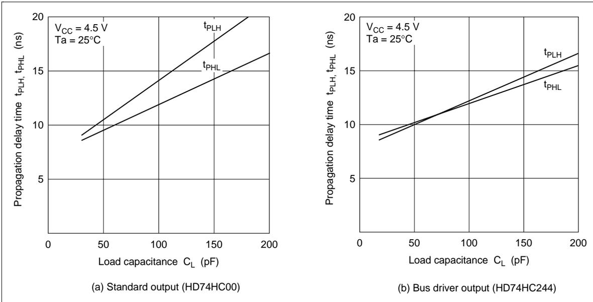
**Figure 11 Propagation Delay Time vs Load Capacitance**
