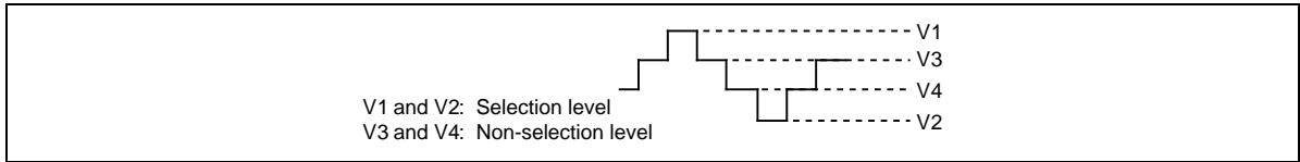
Figure 3 Liquid Crystal Display Drive Level
