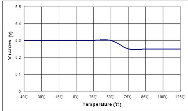
**Figure 17. Latch-Off Threshold Voltage (V<sub>LATCHth</sub>) vs. Temperature**
