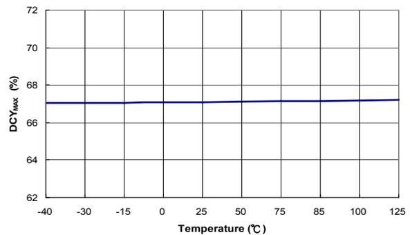
**Figure 13. Maximum Duty Cycle ( $DCY_{MAX}$ ) vs. Temperature**
