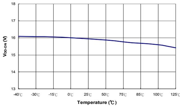
**Figure 8. Start Threshold Voltage ( $V_{DD-ON}$ ) vs. Temperature**
