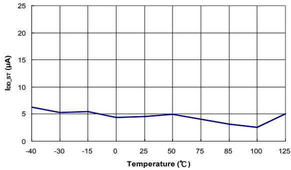
**Figure 6. Startup Current ( $I_{DD-ST}$ ) vs. Temperature**
