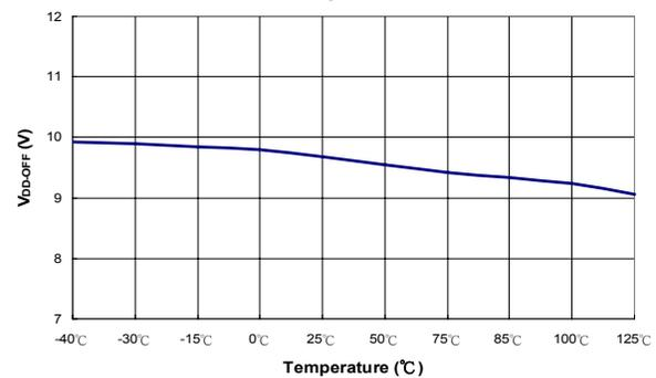
**Figure 9. Minimum Operating Voltage ( $V_{DD-OFF}$ ) vs. Temperature**
