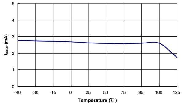
**Figure 7. Operation Supply Current ( $I_{DD-OP}$ ) vs. Temperature**
