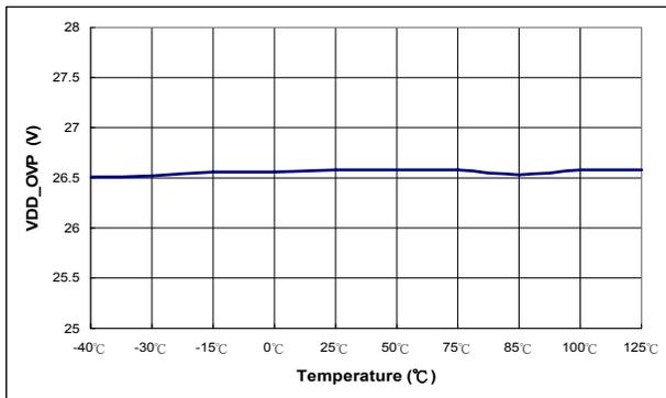
**Figure 18. V<sub>DD</sub> Over-Voltage Protection (V<sub>DD-OVP</sub>) vs. Temperature**
