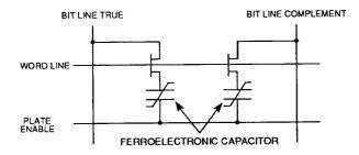
is applied to the ferroelectronic capacitor. The plate enable signal is pulsed to polarize the data in one of the two stable states of the ferroelectric material. The information stored in the polarized capacitor is retained until the next memory reference to this cell without refreshing or maintaining the power supply. Therefore, the FRAM acts as a nonvolatile static RAM.
