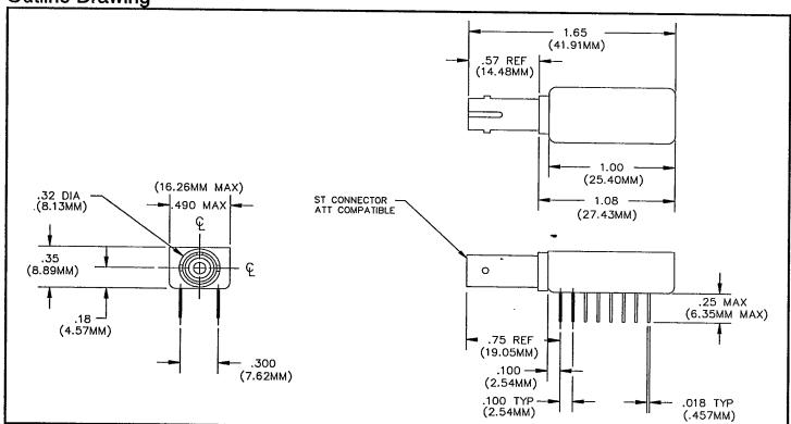
The metal housing is conductive and should be prevented from contacting circuit board traces or the sleeves of low profile screw machine sockets.
