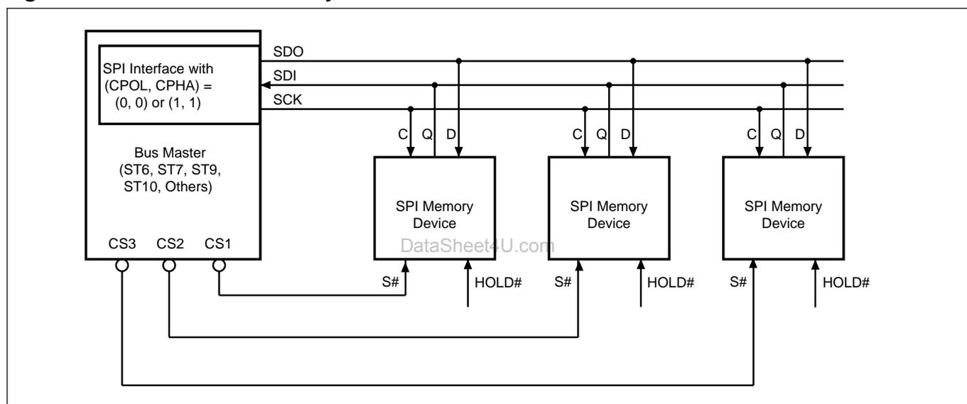
Note: 1. Hold (HOLD#) signals should be driven, High or Low as appropriate.
