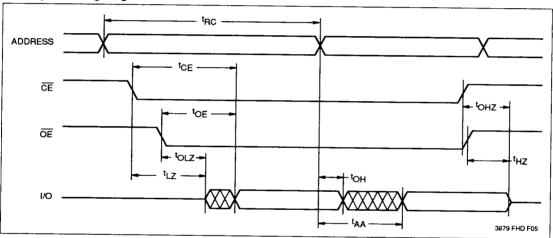
Note: (3) t<sub>LZ</sub> min., t<sub>HZ</sub> min., t<sub>OLZ</sub> min., and t<sub>OHZ</sub> min. are periodically sampled and not 100% teseted. t<sub>HZ</sub> max. and t<sub>OHZ</sub> max. are measured from the point when  $\overline{\text{CE}}$  or  $\overline{\text{OE}}$  return high (whichever occurs first) to the time when the outptus are no longer driven.
