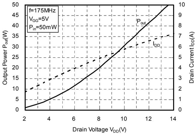
TYPICAL PERFORMANCE ( $T_{case}=+25^{\circ}C$ ,  $Z_G=Z_L=50\Omega$ , unless otherwise specified)
