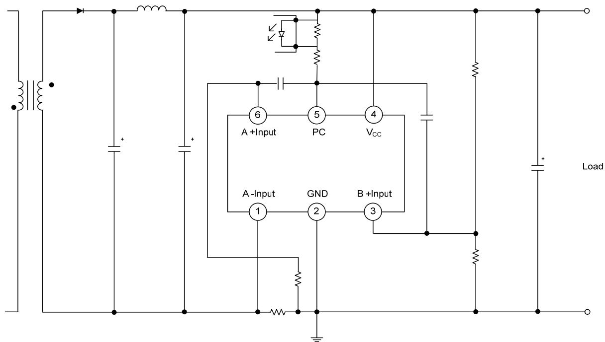
In the above application schematic, the UTC **UM607** is used on the secondary side of a flyback adapter (or battery charger) to provide an accurate control of voltage and current. The above feedback loop is made with an optocoupler.
