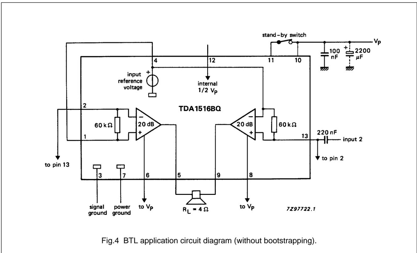
24 W BTL or 2 x 12 watt stereo car radio power amplifier
