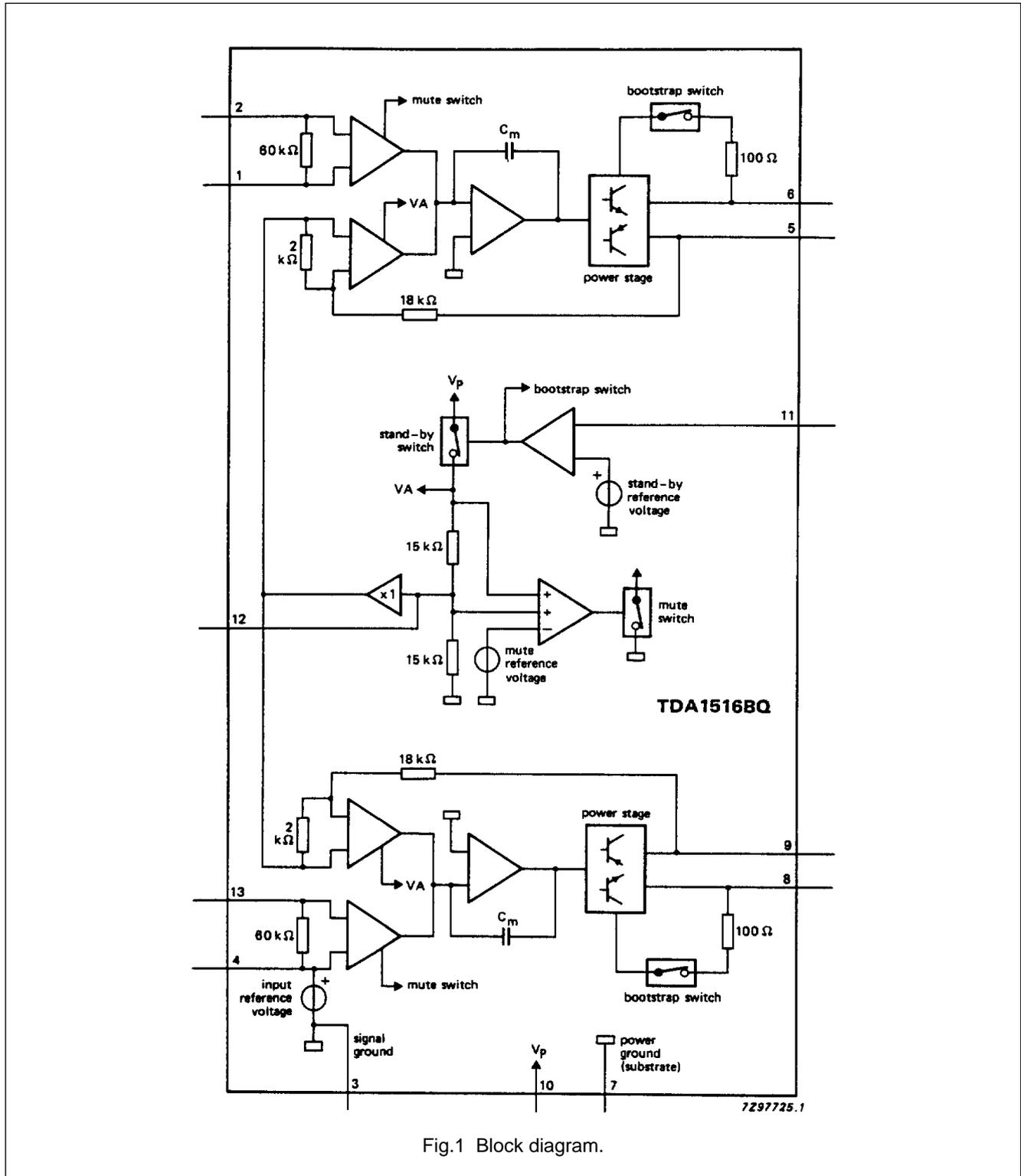
Fig.1 Block diagram.
