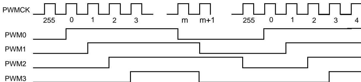
**FIGURE 9. 5 Channel PWM Output Rising Edges Are Separated by One PWMCK**
