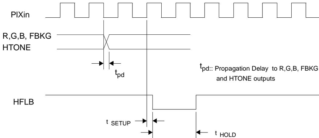
FIGURE 12. Output and HFLB Timing to Pixel Clock
