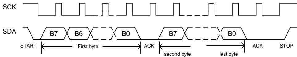
**FIGURE 2. Data Transmission Protocol (I<sup>2</sup>C)**
