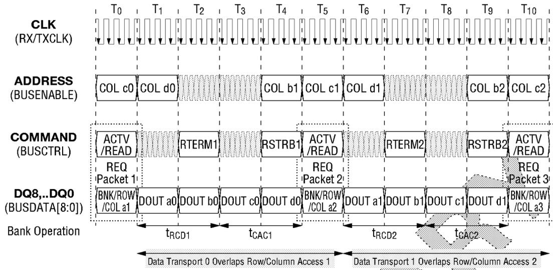
Fig. 5 Interleaved Read Transaction Example
