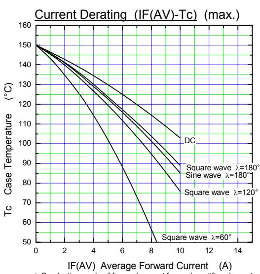
$\lambda$ :Conduction angle of forward current for each rectifier element
