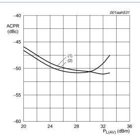
$V_{DS}$  = 28 V;  $I_{Dq}$  = 350 mA;  $f_1$  = 952.5 MHz;  $f_2$  = 957.5 MHz; carrier spacing 5 MHz.
