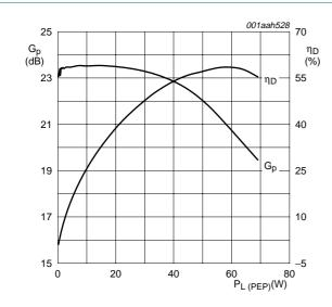
$V_{DS} = 28 \text{ V}; I_{Dq} = 350 \text{ mA}; f_1 = 960 \text{ MHz}; f_2 = 960.1 \text{ MHz}.$
