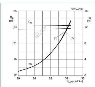
$V_{DS} = 28 \text{ V}; I_{Dq} = 350 \text{ mA}; f_1 = 952.5 \text{ MHz}; f_2 = 957.5 \text{ MHz}; carrier spacing 5 \text{ MHz}.$
