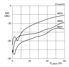
$V_{DS} = 28 \text{ V}; I_{Dq} = 350 \text{ mA}; f_1 = 960 \text{ MHz}; f_2 = 960.1 \text{ MHz}.$
