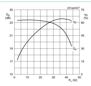
$V_{DS}$  = 28 V;  $I_{Dq}$  = 350 mA; f = 960 MHz.
