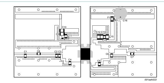
The striplines are on a double copper-clad Taconic RF35 Printed-Circuit Board (PCB) with  $\epsilon_{\text{r}}$  = 3.5 and thickness = 0.76 mm.
