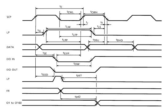
TEST CONDITIONS (1) (Unless Otherwise Noted,  $V_{SS}$  = 0 V,  $V_{DD}$  = 4.5 to 5.5 V,  $V_{CC}$  = 14 to 42 V, Ta = -20 to 75°C)
