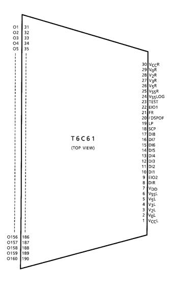
The above diagram shows the pin configuration of the LSI chip, not that of the tape carrier package.
