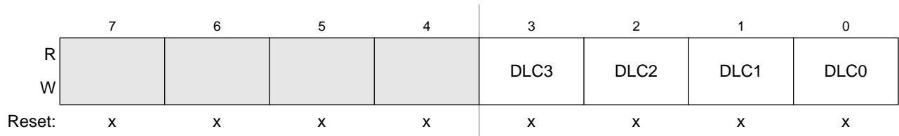
Figure 12-34. Data Length Register (DLR) — Extended Identifier Mapping
