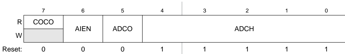
Figure 10-3. Status and Control Register (ADCSC1)
