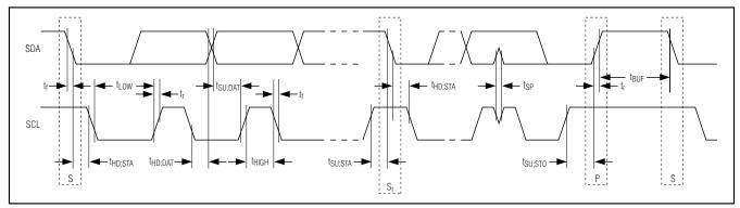
Figure 1. 2-Wire Serial-Interface Timing Diagram
