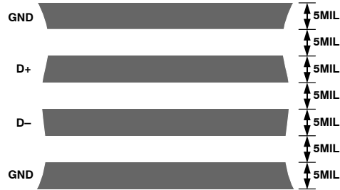
Figure 16. Arrangements of Signal Tracks
