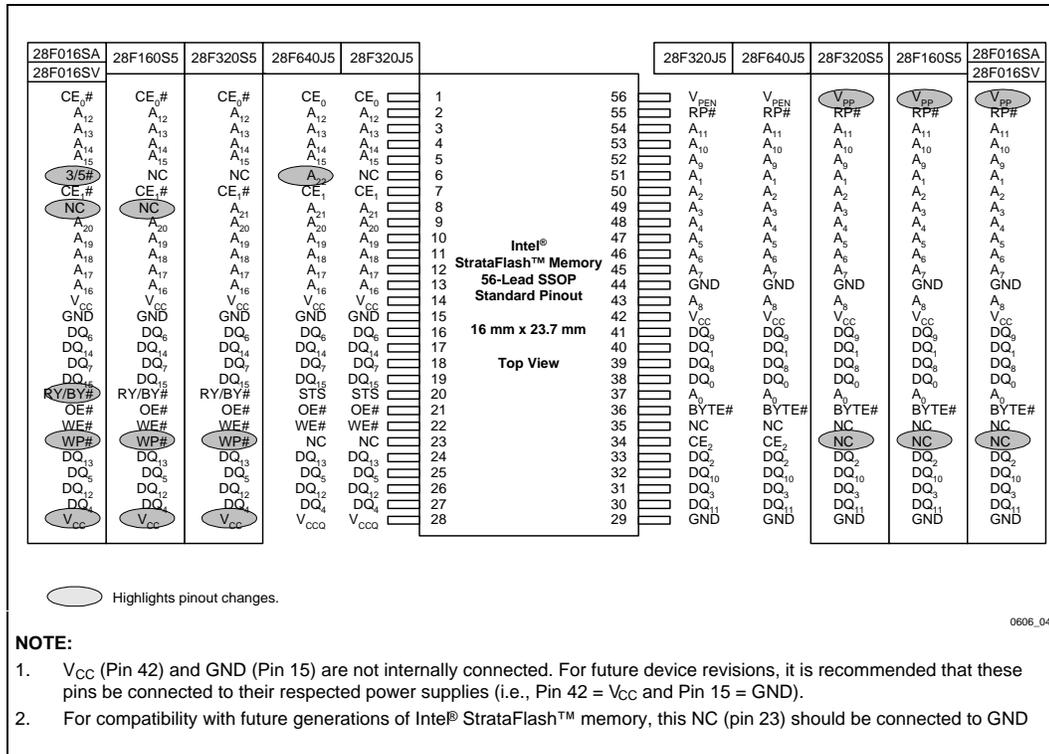
Figure 4. SSOP Lead Configuration (64 Mbit and 32 Mbit)
