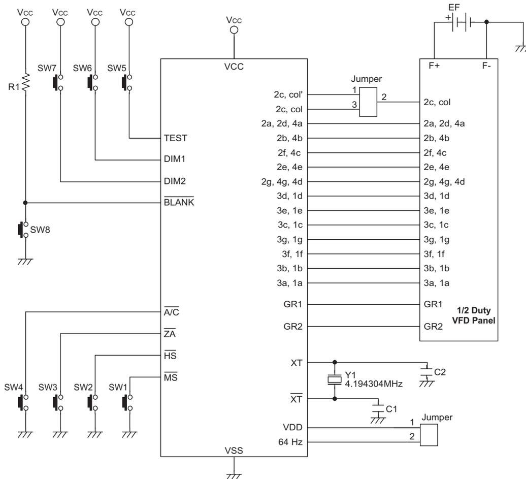
Note: Capacitor C1 and C2 can adjust the accuracy of frequency
