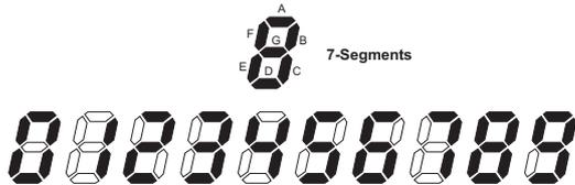
As the device is designed for clock applications, four 7-segment displays are required to display the correct time output. The connections for the grids and segments are shown below, however it should be noted that the fourth segment only requires two of its segments to be driven. Additionally it should be noted that the colon can also be illuminated.
