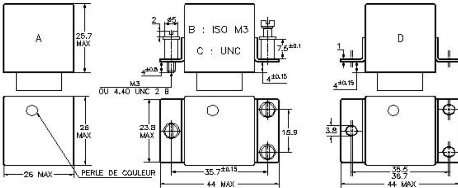
LA FIXATION K PEUT ETRE UTILISEE AVEC LES TYPES DE SORTIES 1 OU 8; ELLE INCLUT LA FOURNITURE DE LA CALE ISOLANTE 10124
