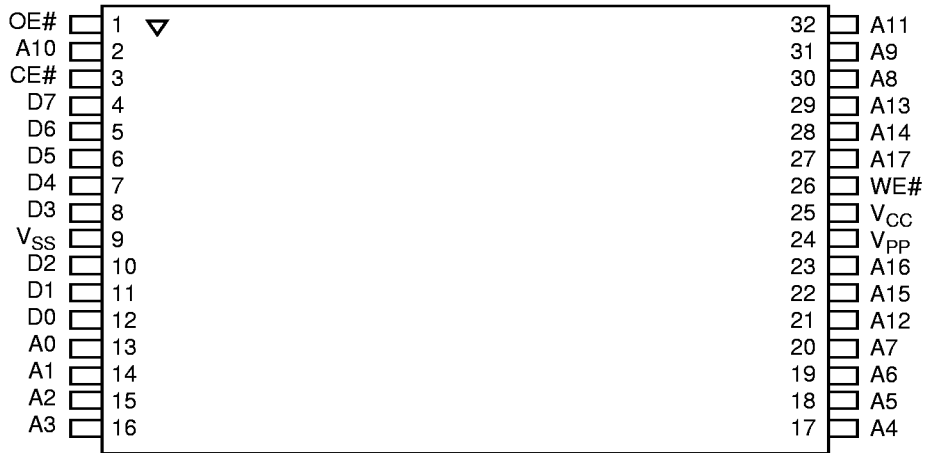
32-Pin TSOP—Reverse Pinout
