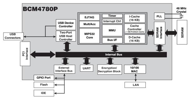
The Broadcom NASoC **BCM4780P** processor is a high-performance, low-power chip designed for entry-level NAS products.
