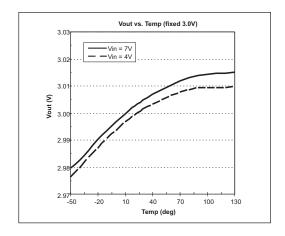
27°C,  $V_{IN}$  = 5.5V,  $I_{O}$  = 0.1mA,  $C_{IN}$  =  $C_{OUT}$  = 1 $\mu F$  unless otherwise specified.
