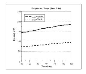
27°C,  $V_{IN}$  = 5.5V,  $I_{O}$  = 0.1mA,  $C_{IN}$  =  $C_{OUT}$  = 1 $\mu F$  unless otherwise specified.
