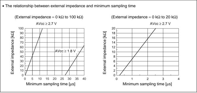
• If the sampling time cannot be sufficient, connect a capacitor of about 0.1 μF to the analog input pin.
