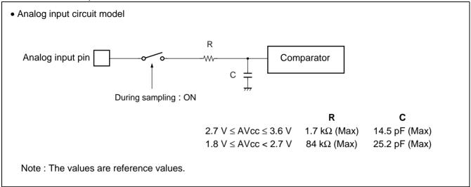
• To satisfy the A/D conversion precision standard, consider the relationship between the external impedance and minimum sampling time and either adjust the resistor value and operating frequency or decrease the external impedance so that the sampling time is longer than the minimum value.
