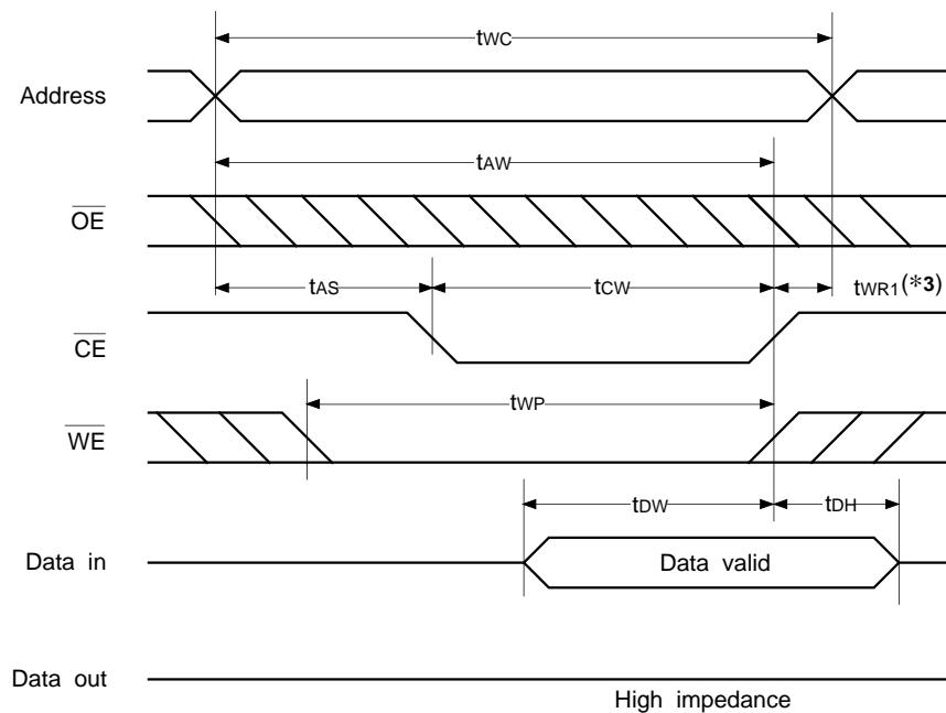
\*1 Write is executed when both  $\overline{\text{CE}}$  and  $\overline{\text{WE}}$  are at low simultaneously.
