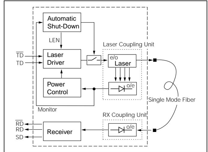
The receiver component converts the optical serial data into PECL compatible electrical data (RD and RDnot). The Signal Detect (SD, active high) shows whether optical data is present<sup>(1)</sup>.
