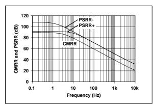
**FIGURE 2-15:** CMRR, PSRR vs. Frequency.
