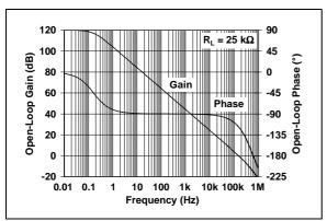
**FIGURE 2-8:** Open-Loop Gain and Phase vs. Frequency.
