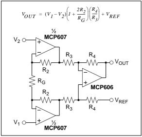
**FIGURE 4-9:** Three op amp Instrumentation Amplifier.
