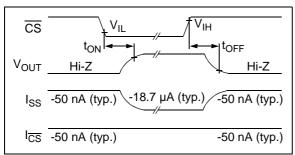
**FIGURE 1-1:** Timing Diagram for the  $\overline{\text{CS}}$  Pin on the MCP608.
