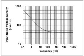
**FIGURE 2-12:** Input Noise Voltage Density vs. Frequency.
