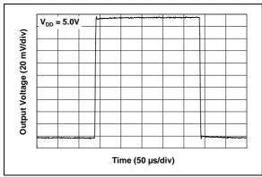
**FIGURE 2-26:** Small-signal, Non-inverting Pulse Response.
