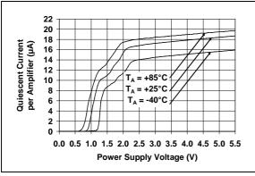
**FIGURE 2-3:** Quiescent Current vs. Power Supply Voltage.
