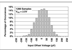
**FIGURE 2-2:** Input Offset Voltage at  $V_{DD} = 2.5V$ .
