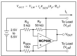
FIGURE 4-5: Low Side Battery Current Sensor.
