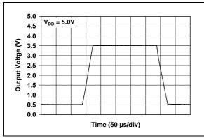
**FIGURE 2-25:** Large-signal, Non-inverting Pulse Response.
