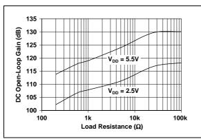
**FIGURE 2-14:** DC Open-Loop Gain vs. Load Resistance.
