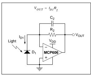
**FIGURE 4-6:** Photodiode (in Photo-voltaic mode) and Transimpedance Amplifier.
