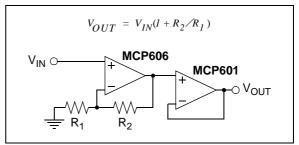
FIGURE 4-10: Precision Gain with Good Load Isolation.
