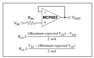
**FIGURE 4-1:** Input Current-Limiting Resistor  $(R_{IN})$ .
