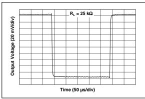
**FIGURE 2-29:** Small-signal, Inverting Pulse Response.
