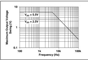
**FIGURE 2-20:** Maximum Output Voltage Swing vs. Frequency.
