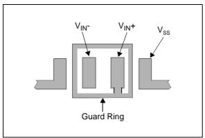
**FIGURE 4-4:** Example Guard Ring Layout for Inverting Gain.
