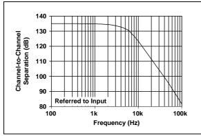
FIGURE 2-9: Channel-to-Channel Separation (MCP607 and MCP609 only).
