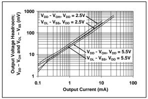
**FIGURE 2-19:** Output Voltage Headroom vs. Output Current Magnitude.
