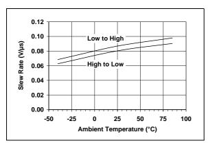
FIGURE 2-21: Slew Rate vs. Ambient Temperature.
