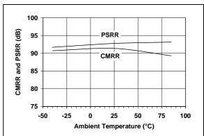
FIGURE 2-18: CMRR, PSRR vs. Ambient Temperature.
