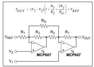
**FIGURE 4-8:** Two op amp Instrumentation Amplifier.
