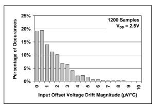
**FIGURE 2-5:** Input Offset Voltage Drift Magnitude at  $V_{DD} = 2.5V$ .
