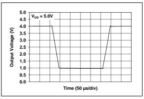
FIGURE 2-28: Large-signal, Inverting Pulse Response.
