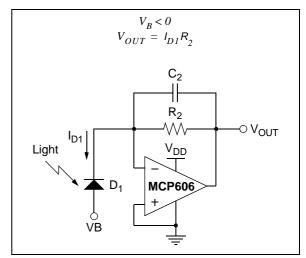
**FIGURE 4-7:** Photodiode (in Photoconductive mode) and Transimpedance Amplifier.
