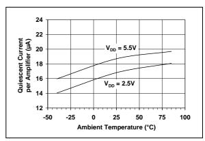
**FIGURE 2-6:** Quiescent Current vs. Ambient Temperature.
