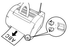
Remove each sheet manually from the face-up delivery slot after it has been printed.
