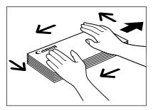
3 Flex the stack on all four sides to remove any stiffness. Check all corners. If the corners are curled, straighten them.
