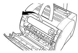
If the leading edge of the paper is visible but has not entered the imaging area, pull the paper forwards and roll it inwards.
