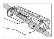
**3** Hold the cartridge, then gently rock it from side to side five or six times to distribute the toner evenly inside the cartridge.
