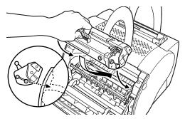
**5** Close the front cover immediately after inserting a cartridge.
