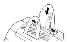
If the flap is along the long edge of the envelope, insert each envelope with the flap at the back and on the right.
