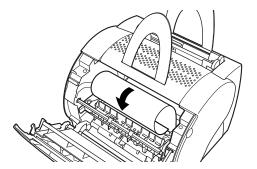
4 Gently pull the rolled up paper out of the printer.
