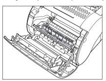
Never touch the high-voltage contact points inside the front cover. This could damage the printer.
