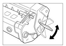
**6** While holding the cartridge firmly with one hand, pull the sealing tape in the direction indicated in the illustration below.
