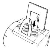
**2** Adjust the paper guides to the sheet of paper.
