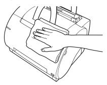
If you use a neutral detergent for cleaning, wipe off the neutral detergent remaining on the printer with a soft cloth, moistened with water.
