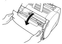
**3** Remove the cartridge by grasping the cartridge's handle and lifting it out of the printer.
