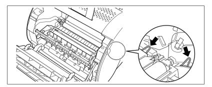
• Remove the jammed paper with the power to the printer still on. If you turn the power off, the data being printing will be erased.
