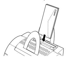
2 Adjust the paper guides to the width of the stack of envelopes.
