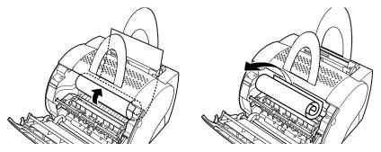
Do not pull the paper upwards from the paper input slot, as this may damage the printer. Gently pull the paper out of the printer.
