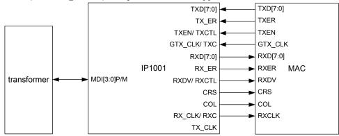
MII is active if pin 15 RGMII\_N/GMII is pulled high and IP1001 islinked at 100M, or 10M.
