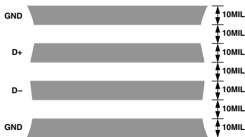
Figure 8. Arrangement of Signal Tracks
