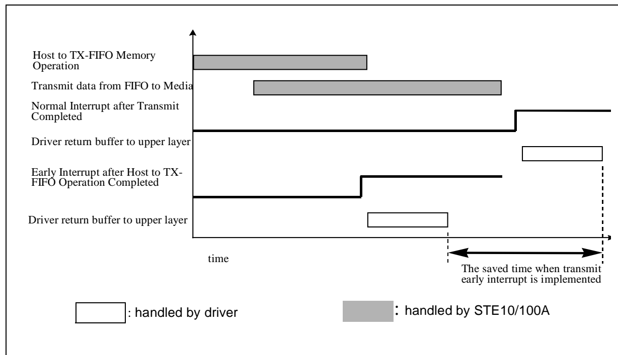
Figure 11. Transmit normal interrupt and early interrupt comparison
