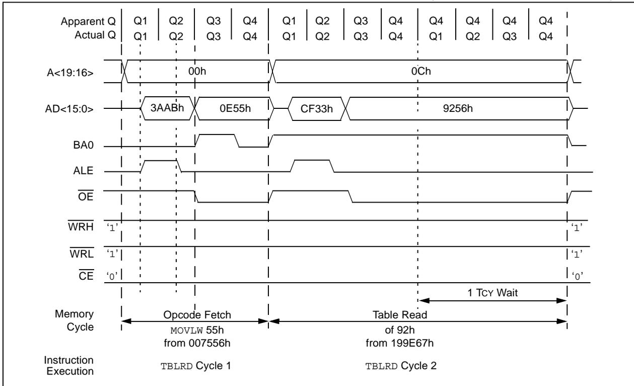
**FIGURE 7-5: EXTERNAL MEMORY BUS TIMING FOR TBLRD (EXTENDED MICROCONTROLLER MODE)**
