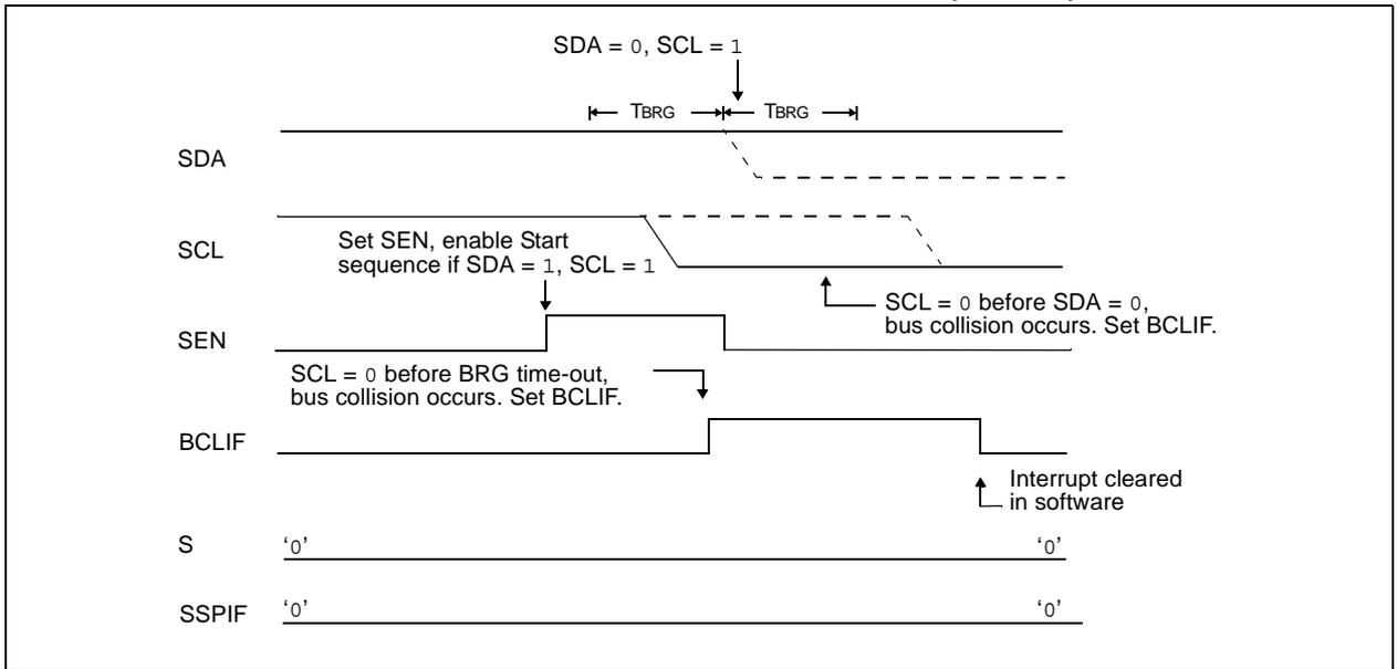
**FIGURE 16-28: BRG RESET DUE TO SDA ARBITRATION DURING START CONDITION**
