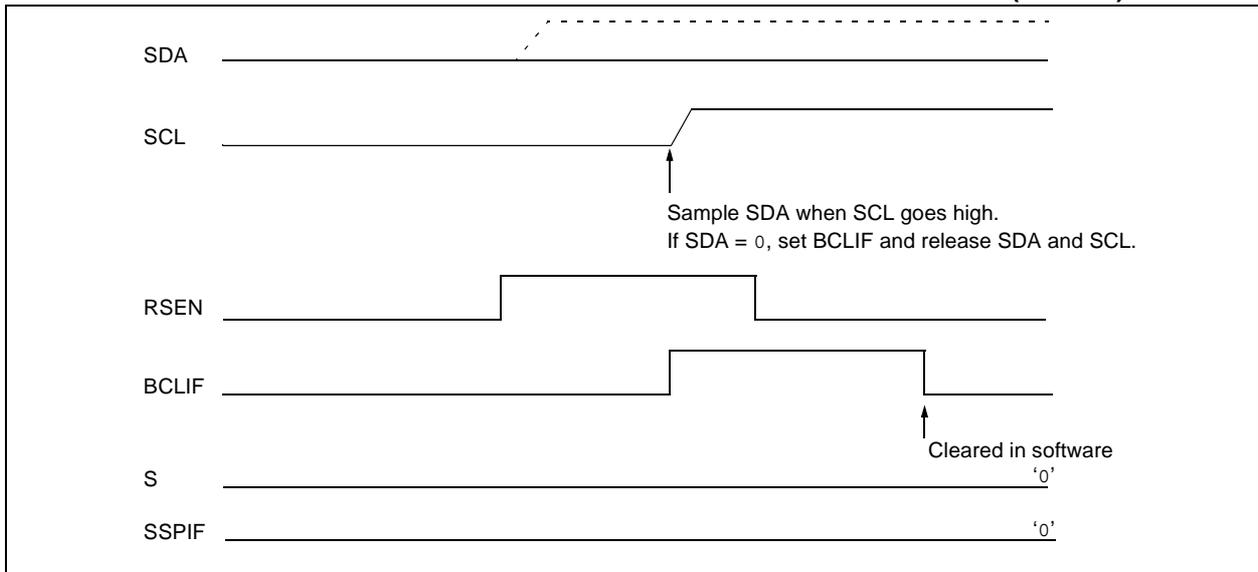
**FIGURE 16-30: BUS COLLISION DURING A REPEATED START CONDITION (CASE 2)**
