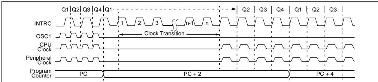
**FIGURE 3-4: TRANSITION TIMING FROM RC\_RUN MODE TO PRI\_RUN MODE**
