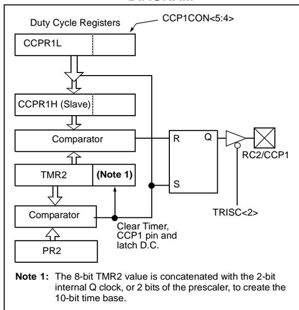
A PWM output (Figure 15-5) has a time base (period) and a time that the output stays high (duty cycle). The frequency of the PWM is the inverse of the period (1/period).
