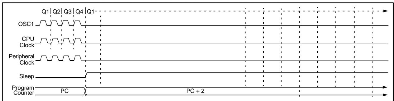
**FIGURE 3-6: TRANSITION TIMING FOR WAKE FROM SLEEP (HSPLL)**
