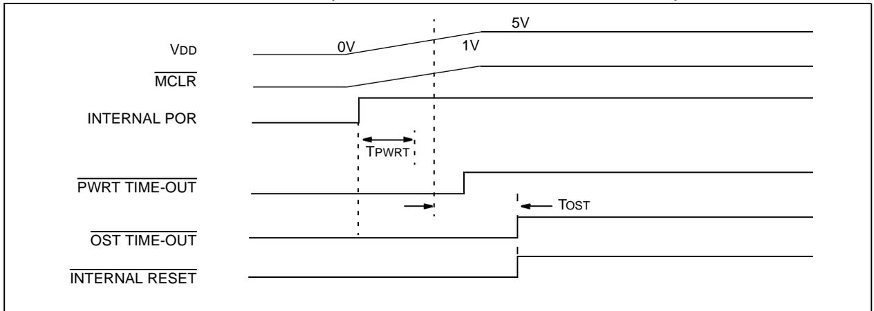
**FIGURE 4-7: TIME-OUT SEQUENCE ON POR W/PLL ENABLED ( $\overline{\text{MCLR}}$  TIED TO  $V_{DD}$ )**
