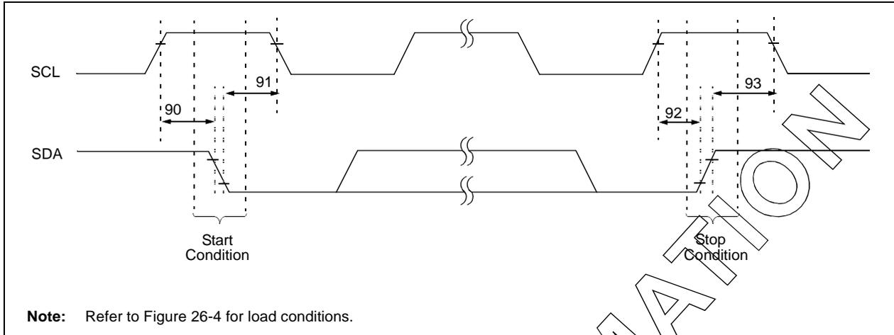
**TABLE 26-19: I<sup>2</sup>C BUS START/STOP BITS REQUIREMENTS (SLAVE MODE)**
