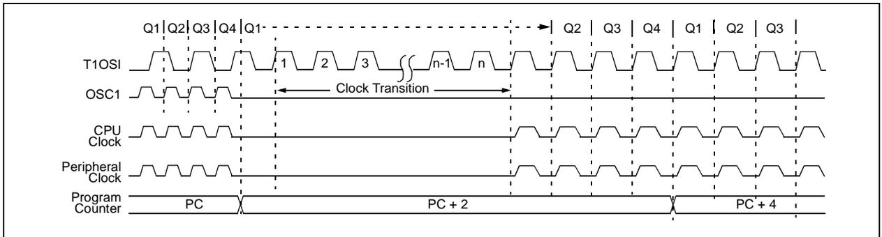
**FIGURE 3-2: TRANSITION TIMING FROM SEC\_RUN MODE TO PRI\_RUN MODE (HSPLL)**
