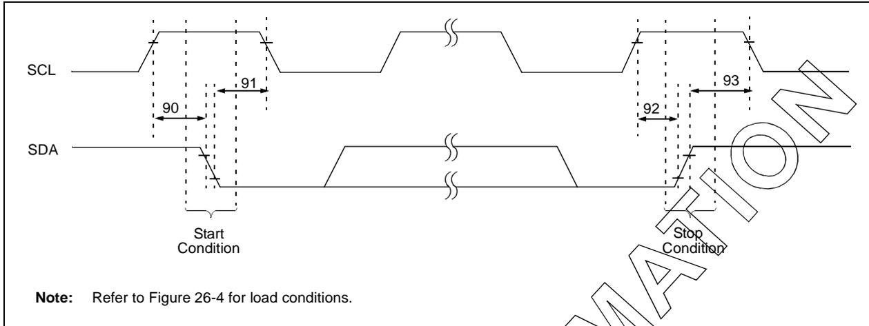
**TABLE 26-21: MASTER SSP I<sup>2</sup>C BUS START/STOP BITS REQUIREMENTS**
