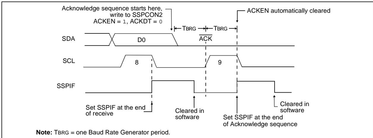
**FIGURE 16-24: STOP CONDITION RECEIVE OR TRANSMIT MODE**
