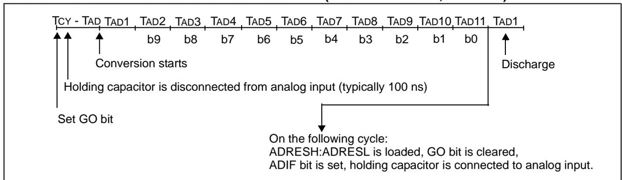
**FIGURE 19-5: A/D CONVERSION TAD CYCLES (ACQT<2:0> = 010, TACQ = 4 TAD)**
