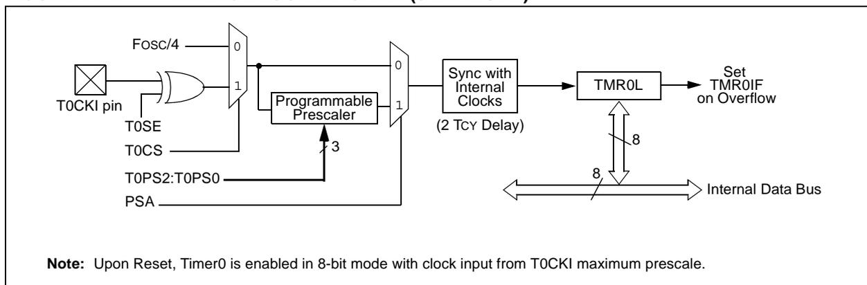
FIGURE 11-2: TIMER0 BLOCK DIAGRAM (16-BIT MODE)
