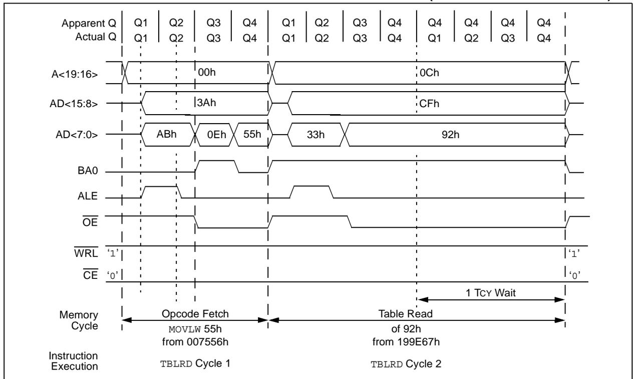
**FIGURE 7-9: EXTERNAL MEMORY BUS TIMING FOR TBLRD (EXTENDED MICROCONTROLLER MODE)**
