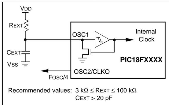
The RCIO Oscillator mode (Figure 2-6) functions like the RC mode, except that the OSC2 pin becomes an additional general purpose I/O pin. The I/O pin becomes bit 6 of PORTA (RA6).
