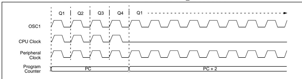
**FIGURE 3-8: TRANSITION TIMING FOR WAKE FROM IDLE TO RUN MODE**
