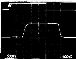
MUX-24 SMALL-SIGNAL SWITCHING WITH FILTERING AND 2.5μs SAMPLE TIME
